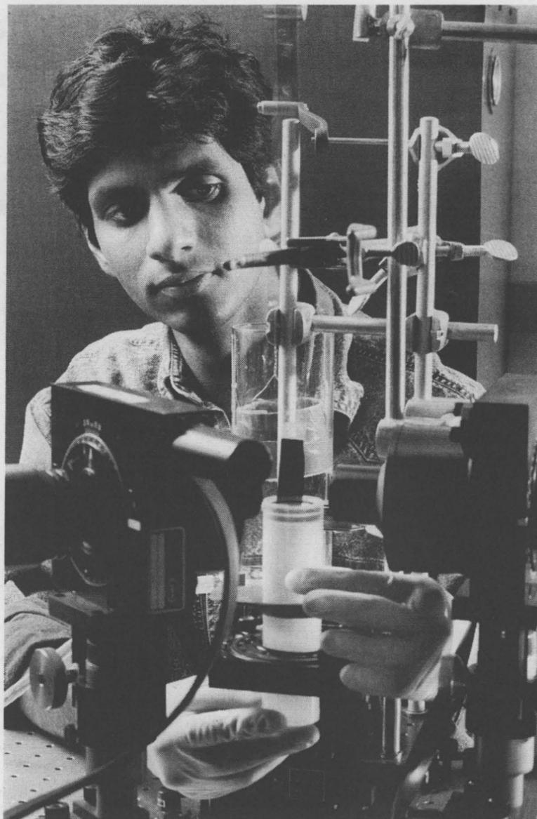
SPONGY AEROFILMS — University of New Mexico graduate student Sai Prakash applies an aerogel film to a substrate using a simple dip-coating procedure. The imaging ellipsometry (laser and camera) equipment in the foreground allows film thickness and refractive index to be measured during film deposition, enabling the researchers to determine how much the aerogel's molecular structure compresses and then springs back when drying stresses are eliminated.
