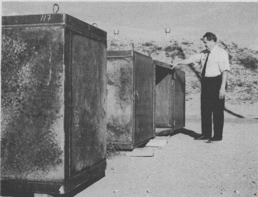
TOUGH CUBES — Lloyd Bonzon (2554) examines explosives storage containers designed for the ECF's on-site storage magazines. Tests have shown that an explosion involving five pounds of explosive material inside one of the cubes will not "sympathetically" detonate explosive materials in a neighboring cube. Each magazine holds up to 24 cubes for a total of 120 pounds of material per magazine. The cubes are made of special fiber-reinforced concrete.
