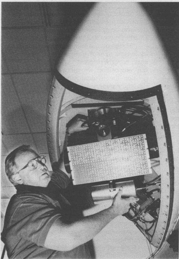
HERE'S LOOKING AT YOU — Sam Bolin of Optical Systems and Image Processing Dept. 9136 adjusts system components inside Sandia's Synthetic Aperture Radar (SAR) pod in a New Mexico lab prior to the recent Florida mission. Pod One, as the 16-ft-long SAR pod is called, contains the radar equipment, video camera, timing and navigation devices, and all necessary data processing, data storage, and power supply equipment.
