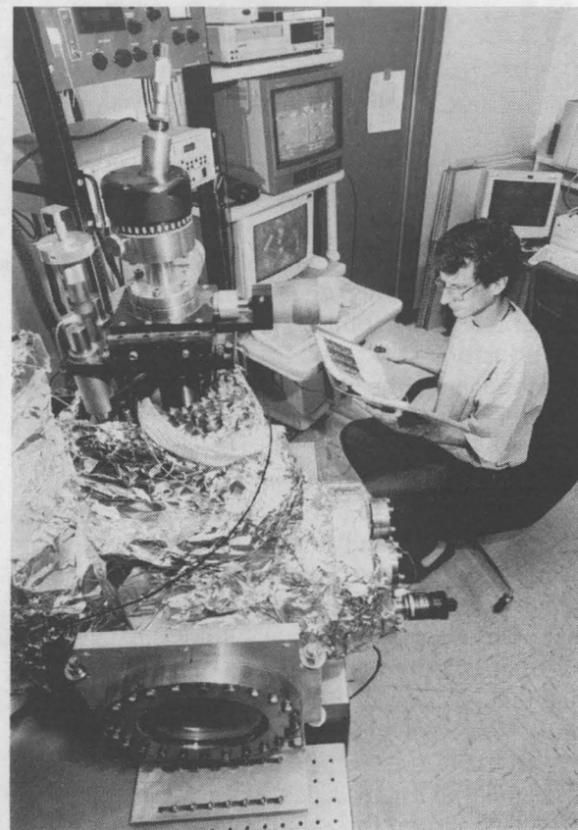
**WATCHING THEM MOVE** — Brian Swartzentruber (1114) at the scanning tunneling microscope he modified to track individual atoms in rapid motion.
