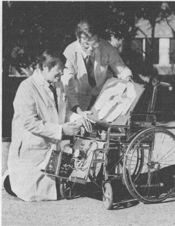
**PRESSURE-FREE** — Gordon Groves (2631, left) and Mark Vaughn (9818) and make adjustments to an "active" wheelchair seat designed to reduce or eliminate the incidence of pressure sores that afflict the wheelchair-bound.
