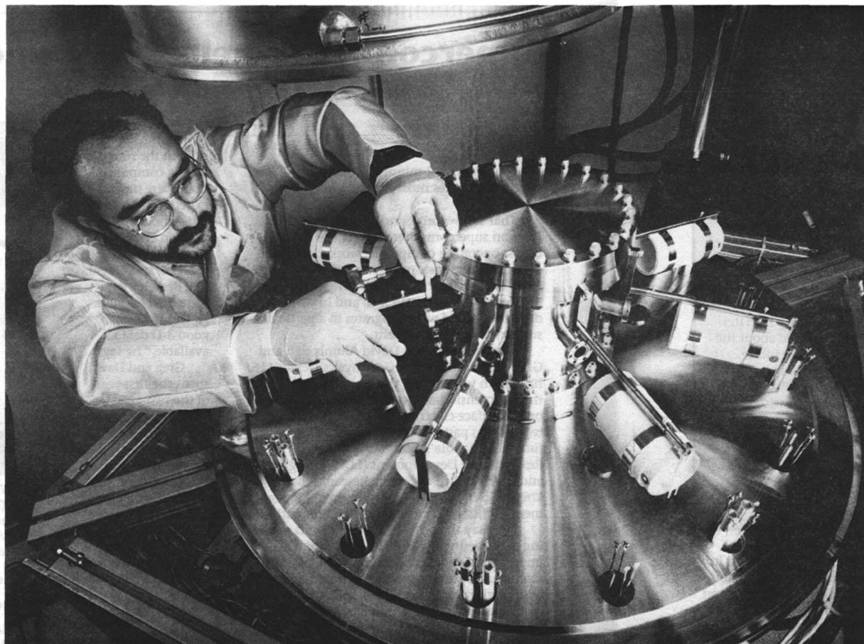
**BAKE STATION** — Mike Lopez (14483) makes adjustments at a neutron tube bake station. The high vacuum bake station is used to thermally treat and evacuate neutron tubes before the final pinch-off (sealing) occurs. The process is critical to ensure the long-term reliability of the tube.
