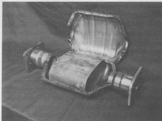
FULL-SCALE prototype catalytic converter.
