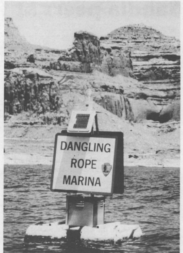
SIGN designating the Dangling Rope Marina is lighted at night with energy collected by a small solar panel. The marina converted its electrical power this summer from a diesel-powered generator to a photovoltaic system with the help of Sandia.
