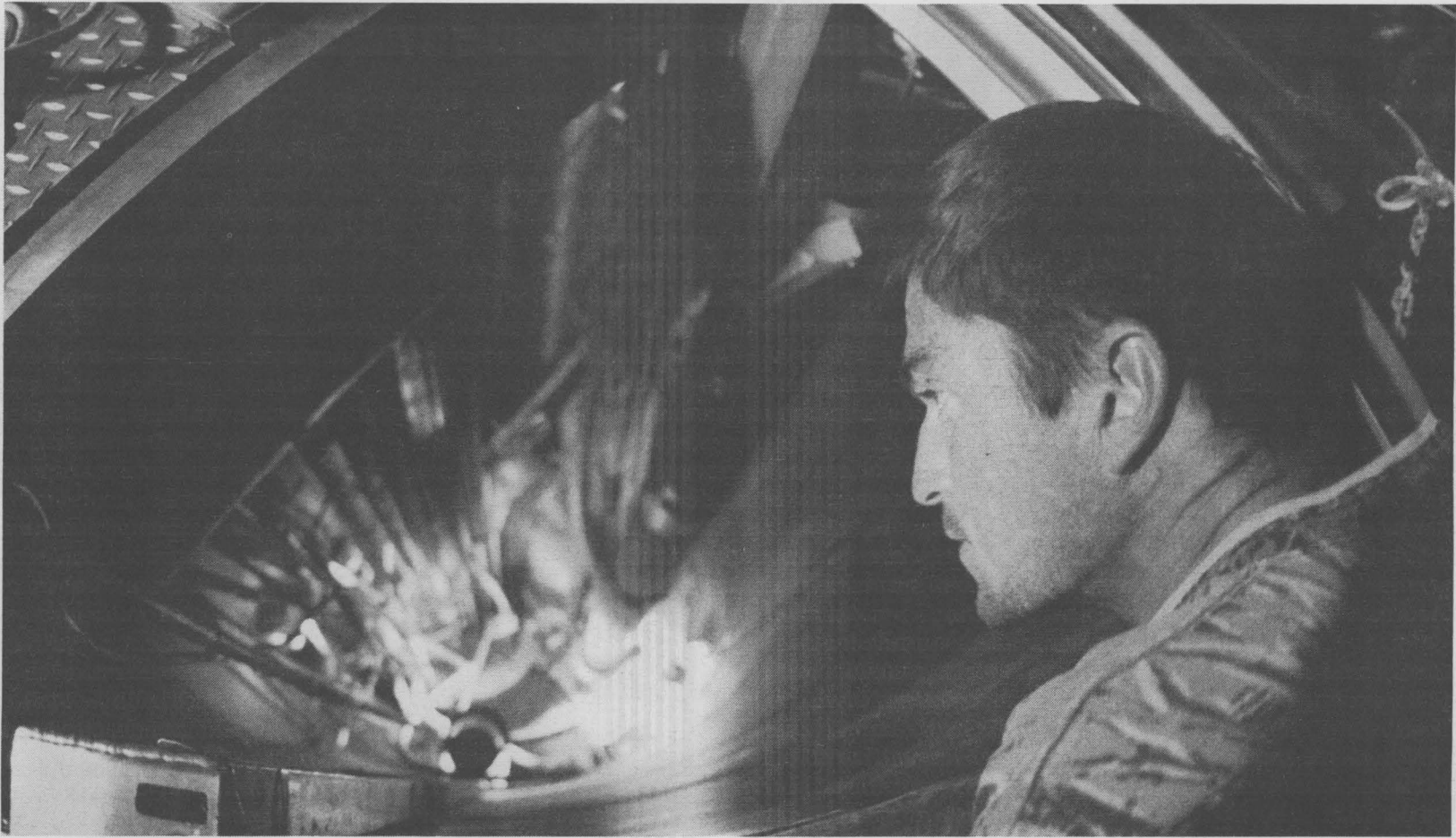
PRODUCTION SITE — Jeff Wemple of Isotope Project and Compliance Initiatives Dept. 9361 peers toward the "hot cell" of the ACRR where targets are placed for irradiation. To make molybdenum-99, sealed target tubes coated on the inside with uranium-235 are placed in the reactor's hot cell and irradiated for several days. (Photography by Randy Montoya)
