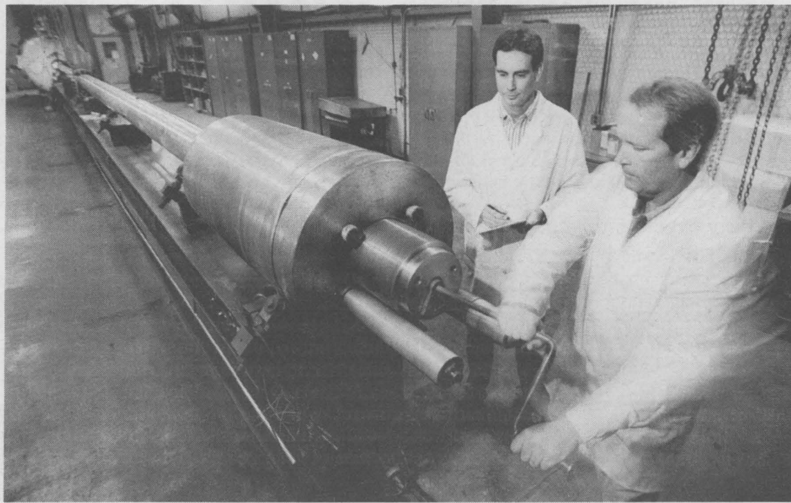
STAR FACILITY WORKERS Clint Hall (9539, left) and Bill Reinhart (1554) install a breech plug in the "Powder Gun" at the STAR facility in preparation for a test. The STAR facility is one of several Sandia test and experimental facilities that have been put on campaign status, meaning they are mothballed most of the time but are available for periodic testing stints, as a result of reduced Laboratories budgets. See story on page 4. (Photo by Mark Poulsen)
