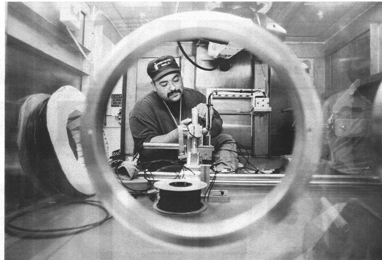
Mike Saavedra (contractor in 9671) hooks up the electrical system for the Automated Component Cleaning (ACC) robot. As part of a project with Allied Signal/Kansas City, Sandia researchers developed a system of automated path planning and programming software that allows the robot to clean a variety of electronic components based on computer-aided design models of the parts and without the use of environmentally harmful solvents.
