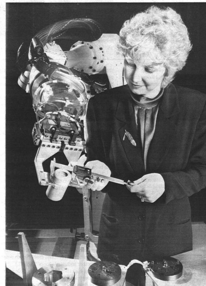
Carla Montoya (9671) measures a mockup of a nuclear weapon gas generator held by Sandia's Automated Gas Generator Disassembly System (AGGDS). The system is currently being installed for disassembly work at the Pantex Plant near Amarillo, Texas.
