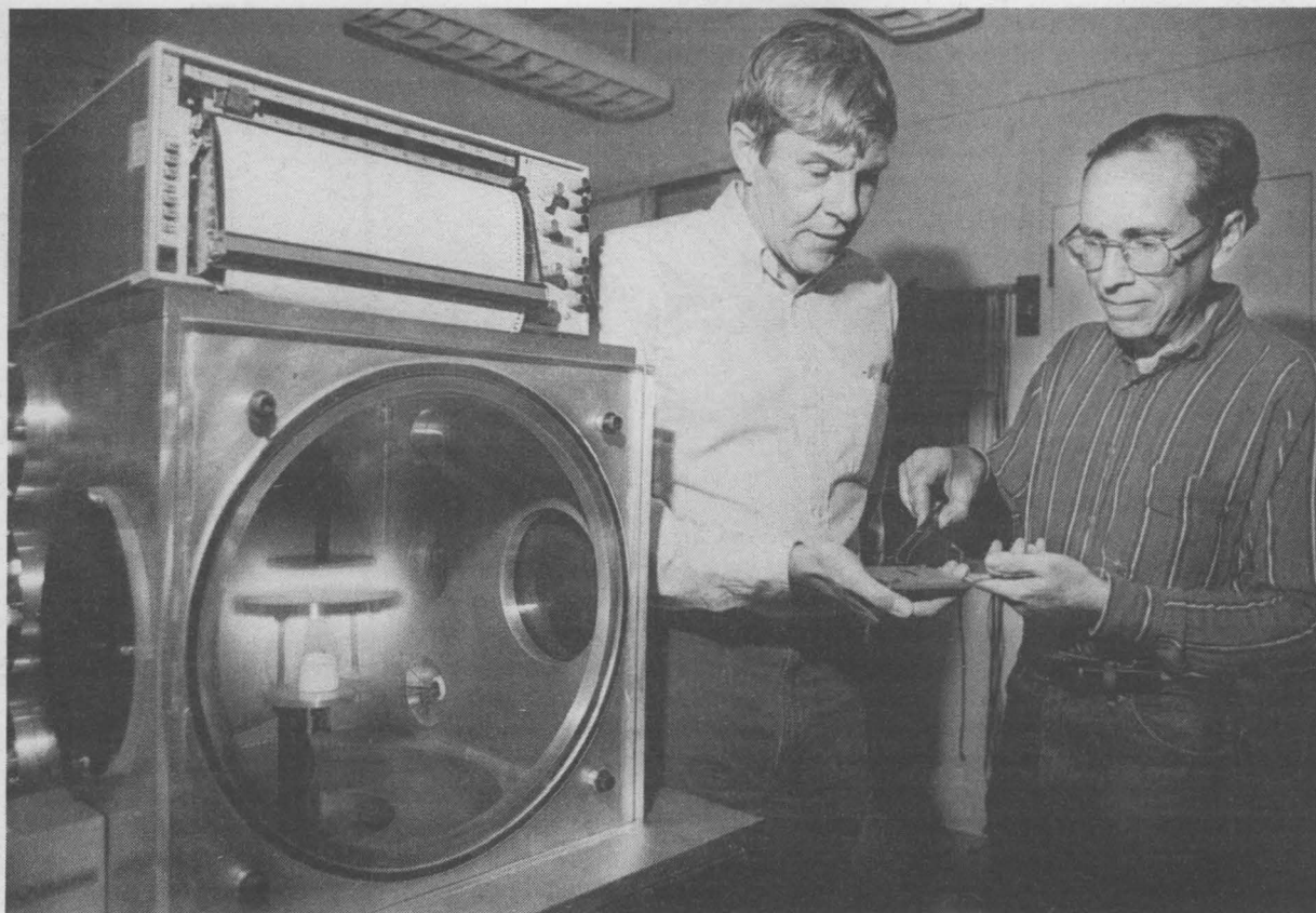
MARS-BOUND — Mike Butler, left, and Rick Buss examine a sample holder used in preparing thin film coatings similar to organic coatings used in the Mars Oxidant Experiment, or MOx. Mike and colleague Tony Ricco conceived of the fiber-optic chemical sensor system used in the MOx experiment, which is the US contribution to the Russian Mars '96 mission. Rick, using this plasma deposition chamber in Bldg. 807, laid down two of the chemical coatings used in the MOx instrument, which was built by NASA's Jet Propulsion Laboratory in Pasadena. (Photo by Mark Poulsen)
