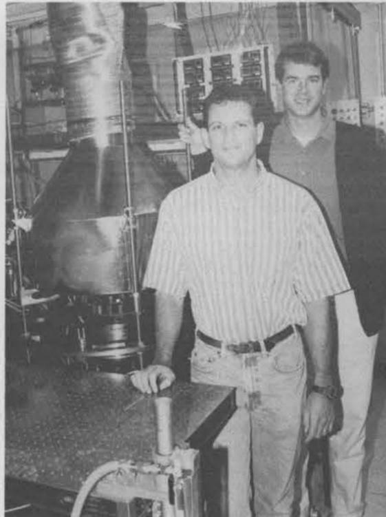
DIAMOND MAKERS — John Wirdzek (left) and David Hahn with the device they used to synthesize sheets of diamond.
