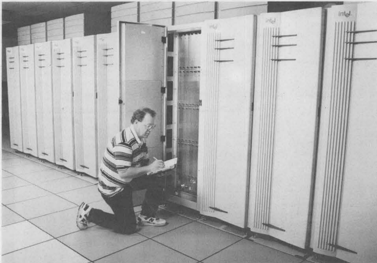
FUTURE SUPERCOMPUTER — James Tomkins (9224), teraflops project manager for procurement, checks the latest shipment of teraflops cabinets from Intel Corp. in Oregon. The teraflops supercomputer, with a computing capacity of 1.8 teraflops, should be up and running at Sandia by late spring. The computer will be used by all three weapons labs for DOE's Accelerated Strategic Computing Initiative. (Photo by Randy Montoya)
