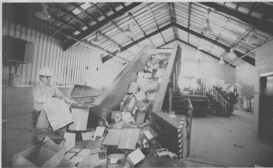
OVER THE TOP — Josue Gonzalez loads cardboard boxes into the Solid Waste Transfer Facility's state-of-the-art conveyor/compactor system. A neat, densely packed one-ton bundle of recyclable material comes out at the other end.
