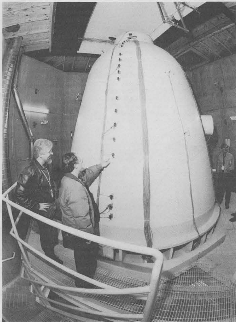
HANDLING THE PRESSURE — Sandia engineers Mike Hessheimer, left, and Vincent Luk, both of International Nuclear Safety Dept. 6403, check out a scale model of a nuclear reactor steel containment vessel prior to a major pressurization test last week. Mike and Vince are part of a Sandia team that is conducting a series of containment-vessel tests for the US Nuclear Regulatory Agency and the Nuclear Power Engineering Corporation of Japan. (Photo by Mark Poulsen)
