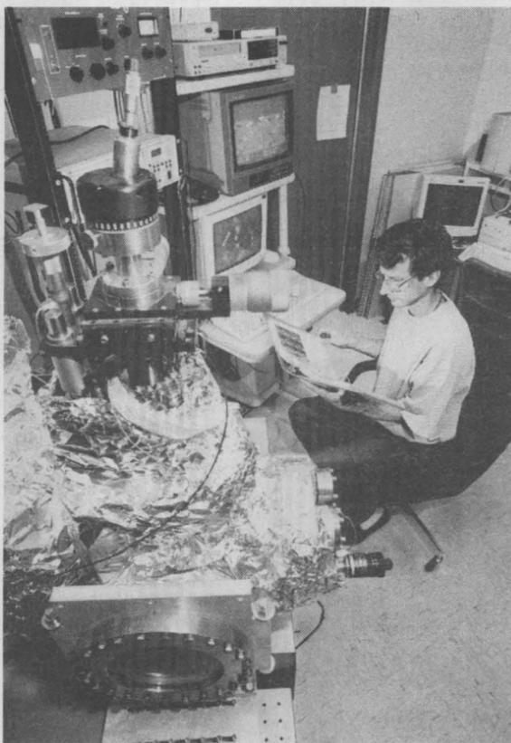
**ATOM TRACKER** — Brian Swartzentruber (1114) watches atoms move using the scanning tunneling microscope he modified to track individual atoms in rapid motion. (Photo by Mark Poulsen)
