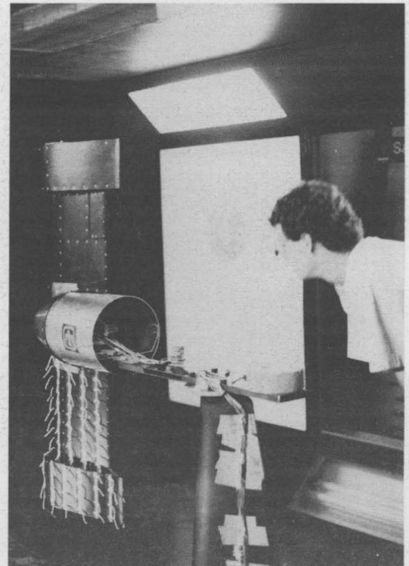
GETTING READY — Doug Parker prepares the radiometer for a wind tunnel test. The instrument mounts onto the wing of an unmanned aerial vehicle to measure solar radiation from the ground and sun.
