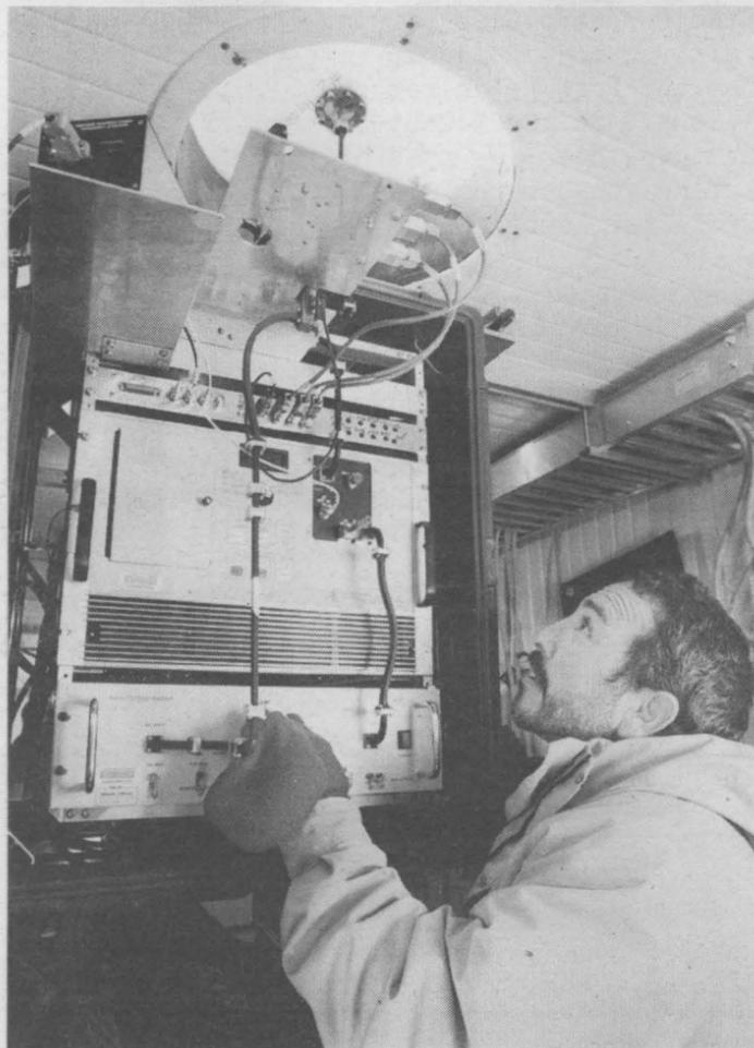
CLOUD WATCHER — Mark Aguilar (6612) makes adjustments to a cloud radar instrument in the Portable Arctic Atmospheric Radiation and Cloud Station — or PAARCS — during predeployment testing and integration at Sandia. The PAARCS will be stationed aboard an icebreaker in the Beaufort Sea north of Barrow, Alaska, for a 13-month drift amidst the arctic ice. (Photo by Mark Poulsen)
