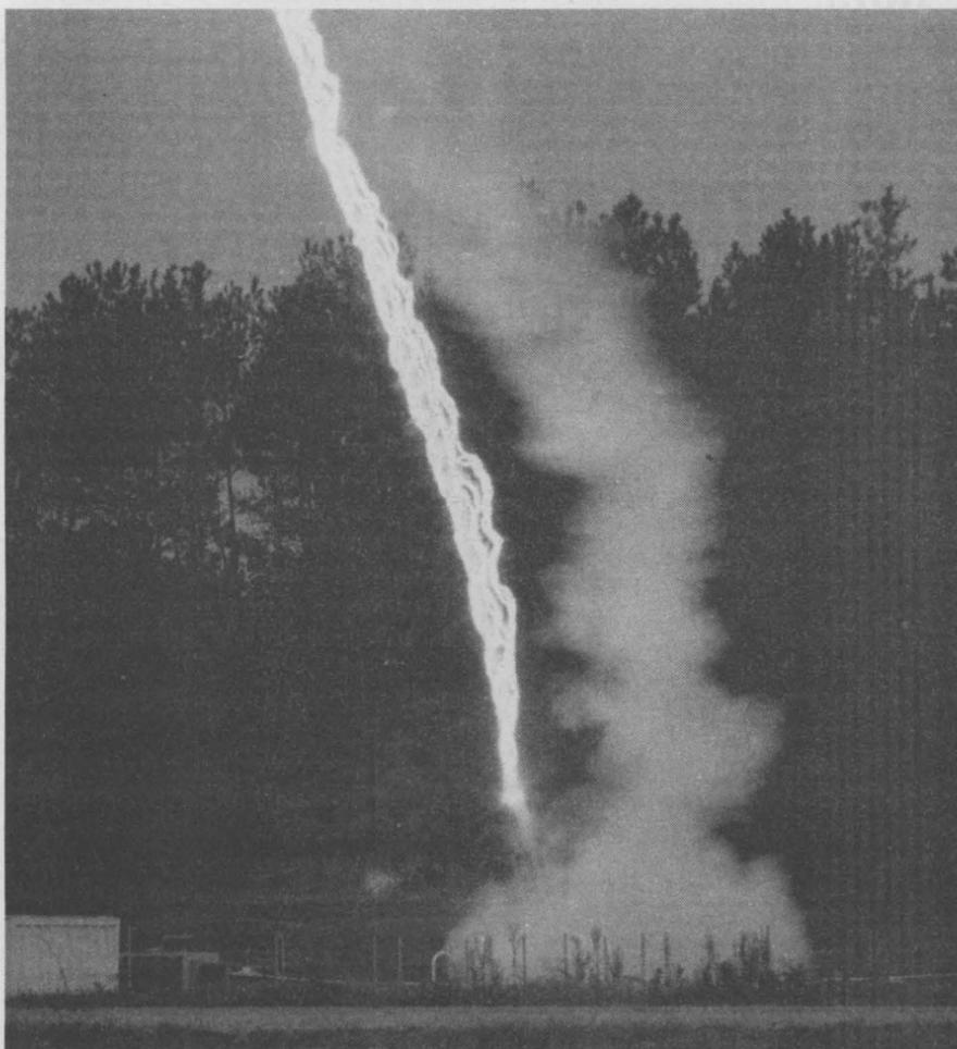
MULTIPLE-STROKE FLASH photographed during a 1993 rocket-triggered lightning test at Ft. McClellan, Ala., aimed at measuring electromagnetic fields on the ground near the flash. The appearance of multiple strokes in the time-exposed photograph is a result of wind drifting particles in the plasma column to the right.
