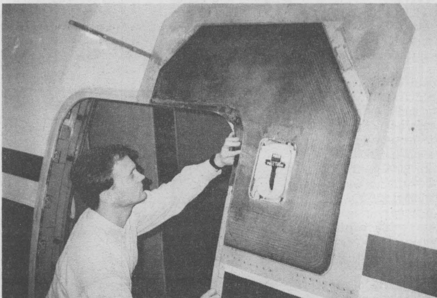
FINISHED PRODUCT — Dennis Roach inspects the L-1011 composite door corner reinforcement prior to application of the Delta paint scheme in February. Edges of the doubler's plies can be seen tapering toward the center. Each successive ply is cut slightly smaller than the last, which helps prevent delamination.
