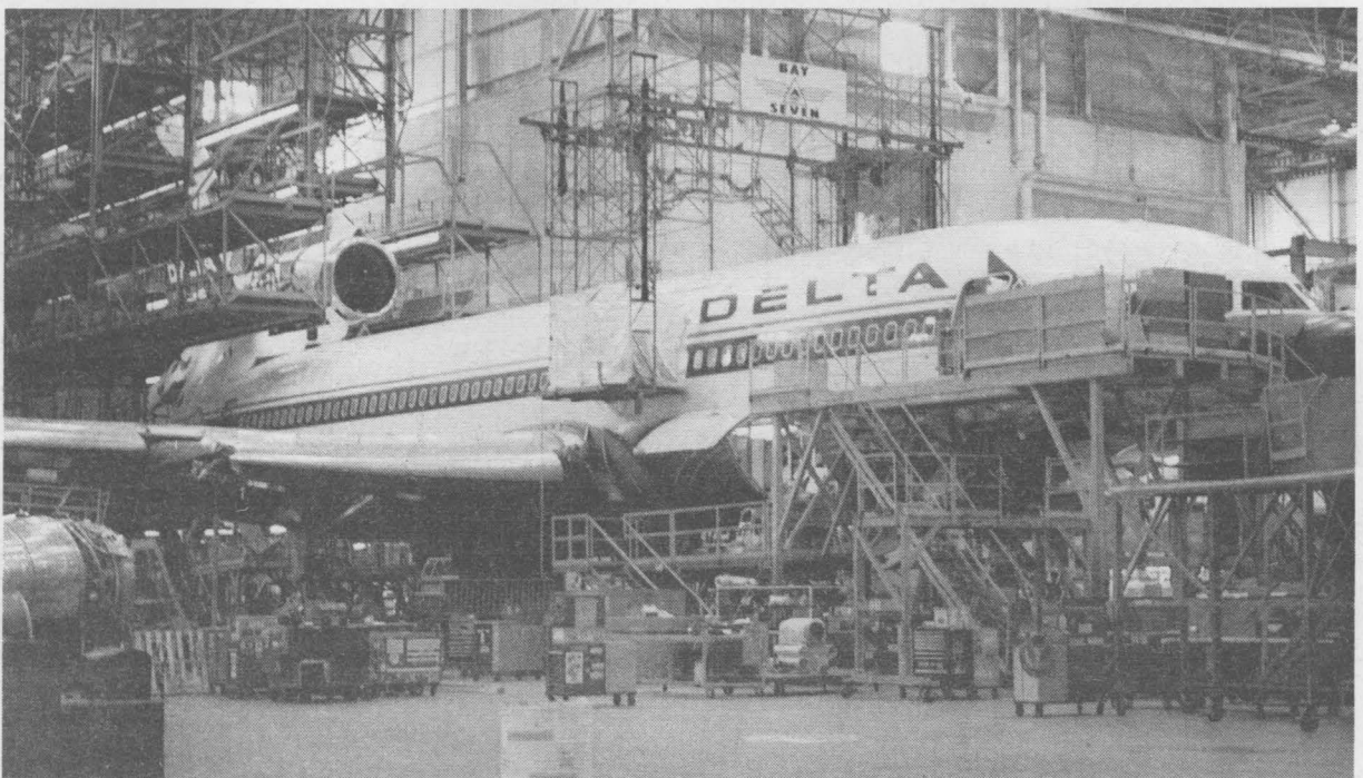
NEW REPAIR TECHNIQUE — During a heavy-maintenance visit at Delta Airline's Technical Operations Center in Atlanta in February, this L-1011 was fitted with a new type of fuselage patch called a bonded composite doubler. The doubler was installed near the right-side access door, seen here cloaked behind a plastic tarp. The new technique was developed at Sandia's Airworthiness Assurance Nondestructive Inspection Validation Center.
