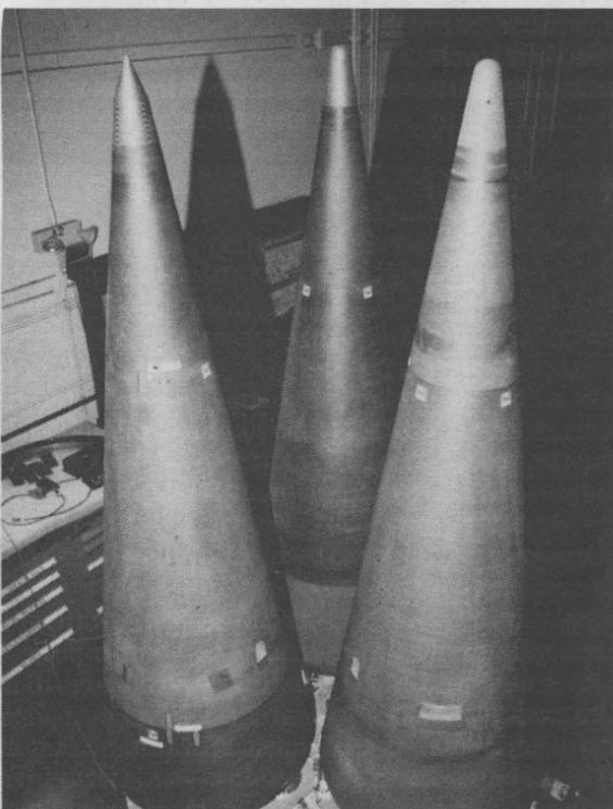
REENTRY TRIO — Three Mk12A reentry vehicles were used in the May 21 operational test. The experimental ultra-high temperature ceramic nose tip, with a sharper point, rode on the RV at left. The other two RVs had standard blunted carbon-carbon nose tips. The photo was taken at Vandenberg prior to launch.
