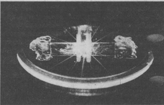
LAB ON A CHIP COMES CLOSER — A biocavity laser — a VCSEL capped by a glass plate enclosing a blood sample, all about the size of a quarter — is excited by a pump laser in Paul Gourley's lab in Bldg. 897. The VCSEL device can produce information about the state of millions of blood cells in a few minutes.
