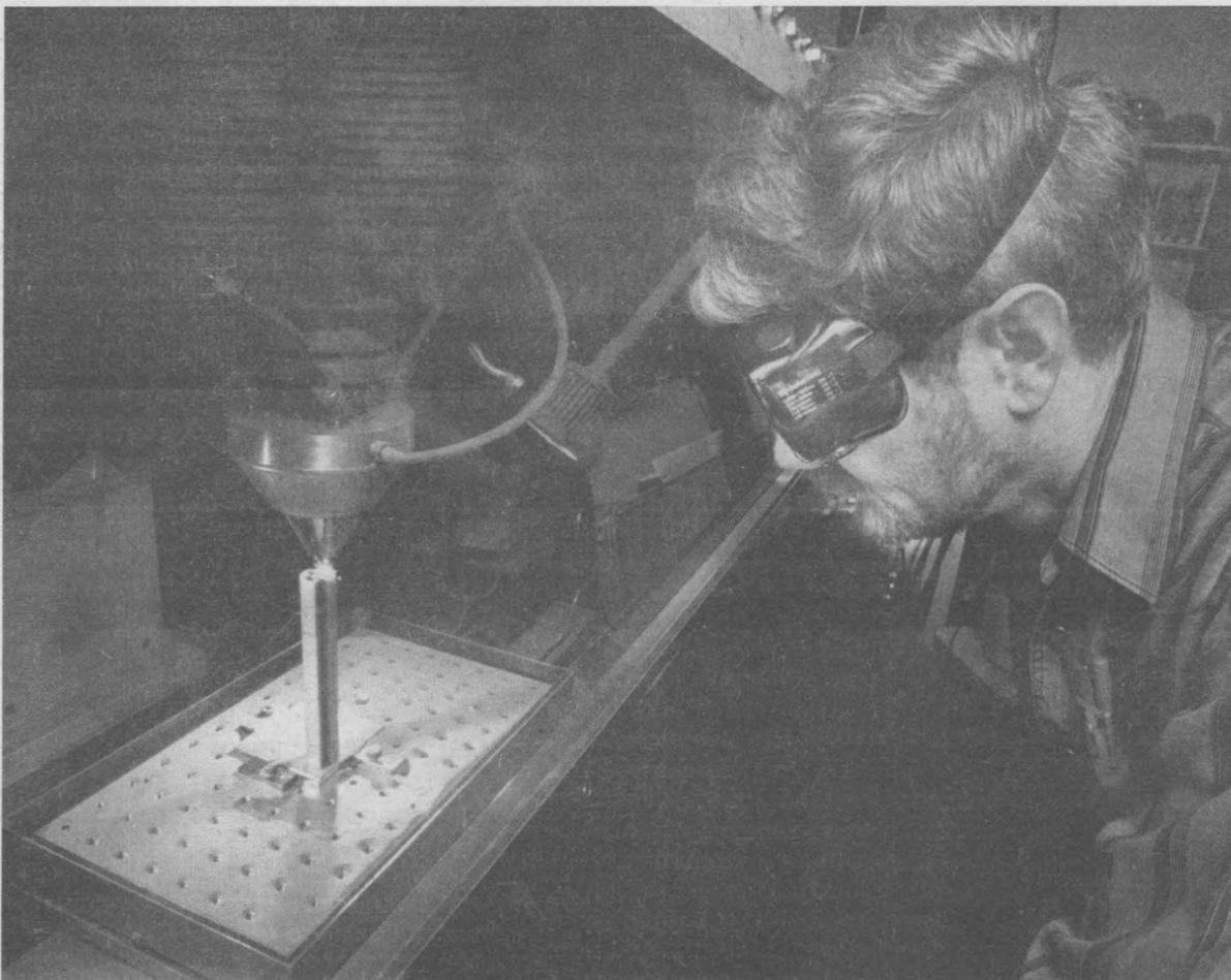
LASER SHAPING — Researcher Lane Harwell (1484) makes an 11-inch-high mini-skyscraper of the T-bird emblem using Sandia's Laser Engineered Net Shaping technique. Ten companies are teaming with Sandia in a two-year, \$3 million cooperative research and development agreement to commercialize the technology.
