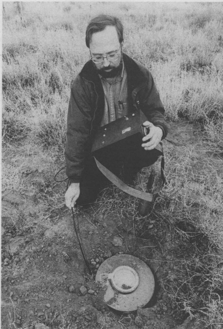
MINE SNIFFER — Phil Rodacy (1552) demonstrates a mock chemical sensing detector on an antitank mine in the makeshift minefield in Tech Area 3. The final field-ready sensor probably will look similar to the mock detector and will be easy to use. (Photo by Randy Montoya)
