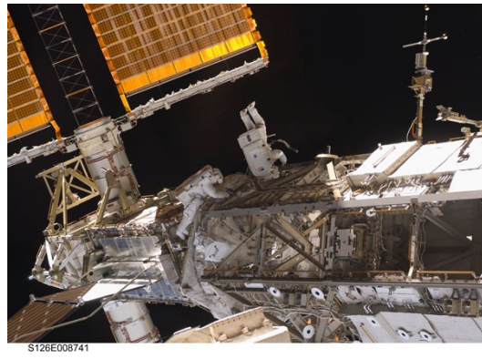
S126-E-008741 (20 Nov. 2008) --- Stefanyshyn-Piper (left) and Kimbrough during EVA2 continue removing debris and applying lubrication around starboard SARJ.
