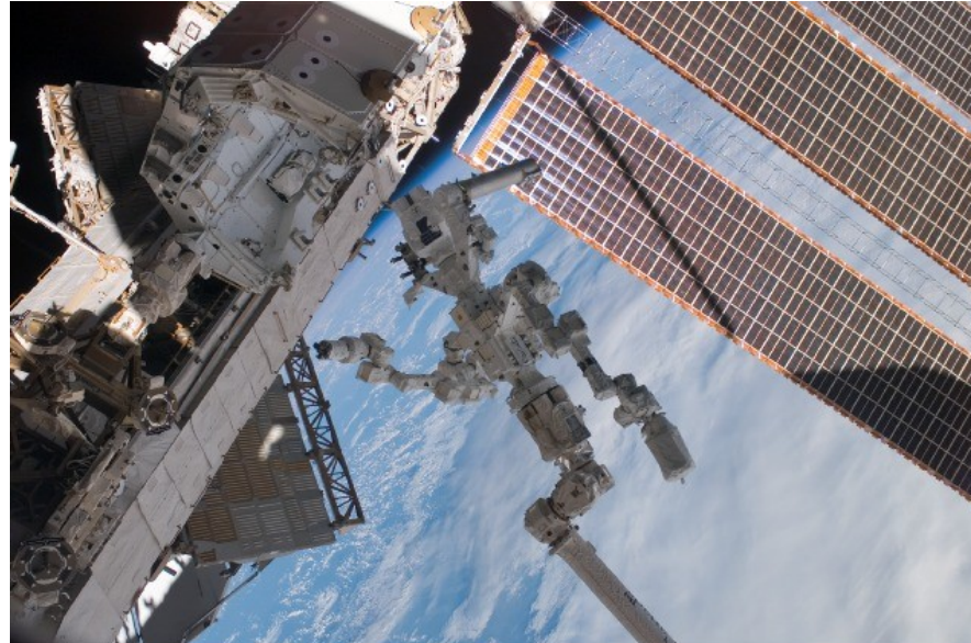
S123-E-007088 (18 March 2008) --- Canada's two armed robot, Dextre, is shown in the grasp of the station's robotic Canadarm2.
